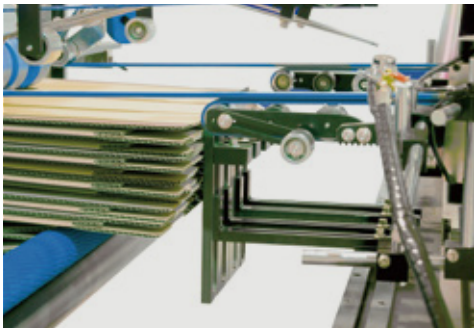
堆疊拍齊裝置 (需搭配-擺臂式氣壓輸送機) The Down Stacking with Square Device (It shall work with Air Pressure Conveyor with Swing Arm.)
