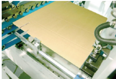
壓著部-枚葉矯正裝置 Alignment Device at Trombone Section
