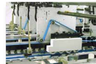
糊帶壓輪 Pressing wheels for Gluing Flap
